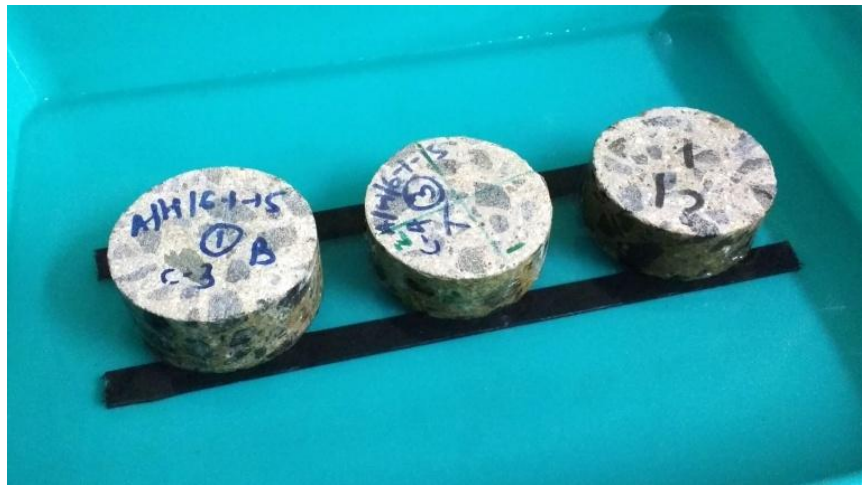
Figure 3.18. Sorptivity test on concrete specimens
