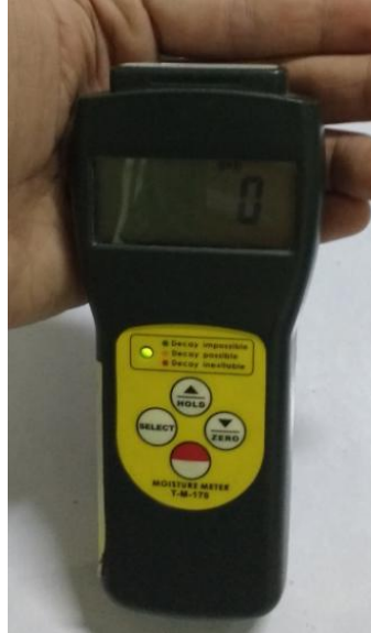
Figure 3.23. Hand-held surface moisture meter used in this study
