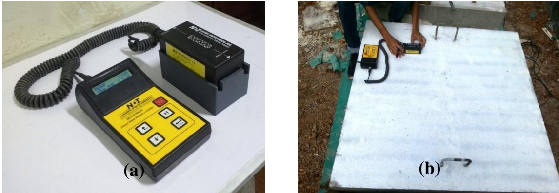
Figure 3.22. (a) Cover meter and its components and (b) rebar detection on field specimen using cover meter
