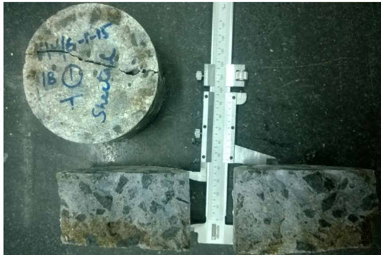
Figure 3.21. Penetration of chlorides into concrete seen as a white precipitate of AgCl on the split face of the specimen
