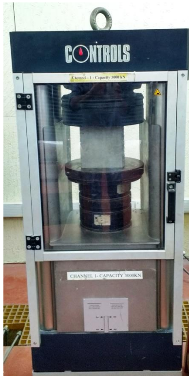
Figure 3.10. Compression testing of cube specimen
