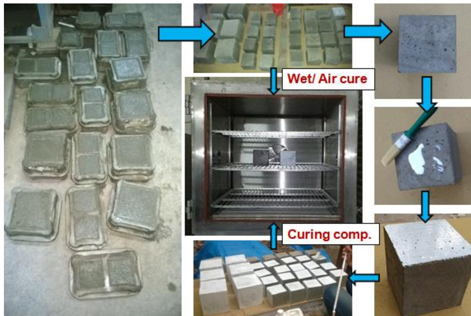
Figure 3.3. Application of curing compound on the cube specimens
