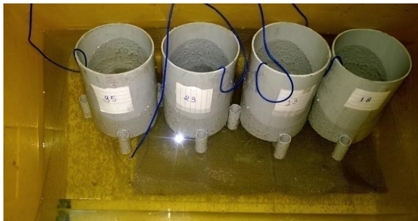
Figure 3.20. RCMT test setup that was used in this study
