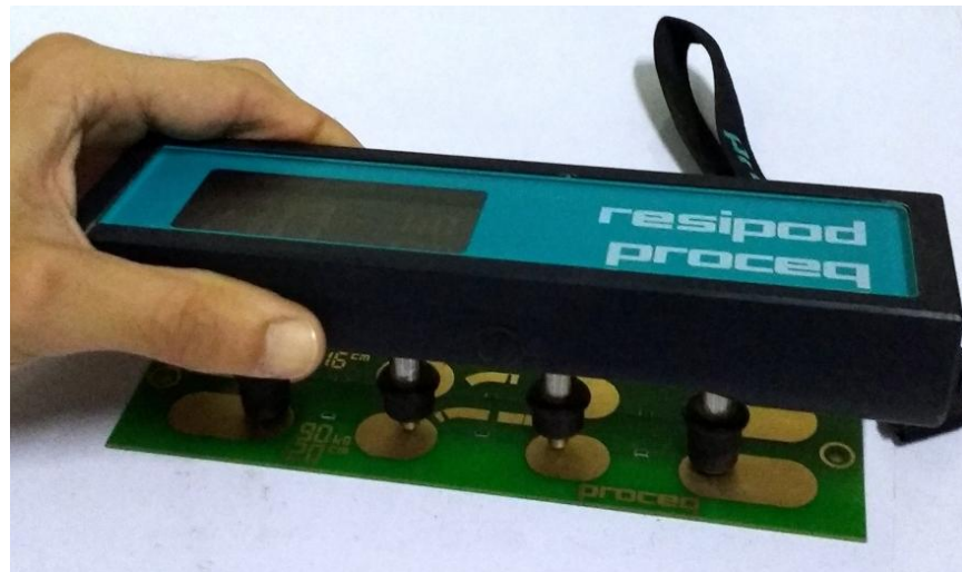
Figure 3.25. Surface resistivity instrument used in this study with the calibration strip
